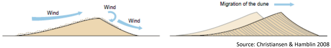
Figure 3: Diagram showing the formation of cross-bedding by dune migration.
