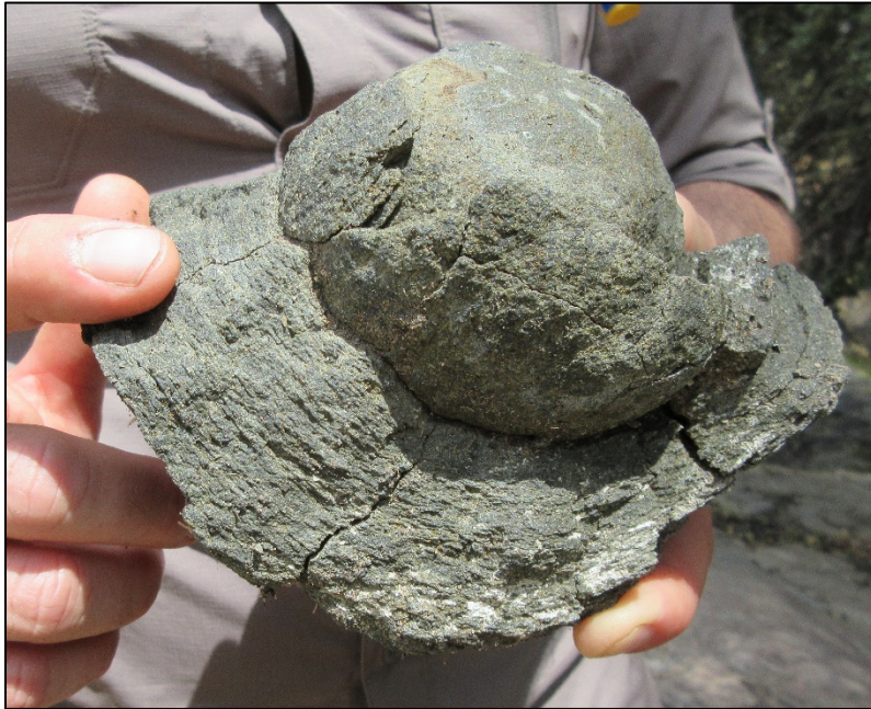
Figure 11: An example of ‘onion-skin’ weathering in Lebombo basalt, showing a rounded core surrounded by several concentric layers.
